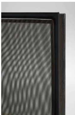
Fig. 23 Moiré effect in insulating glass unit
